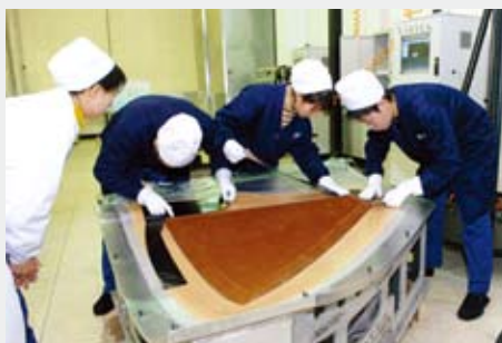
Workers at Harbin making material for wing-to-body fairing panels.
