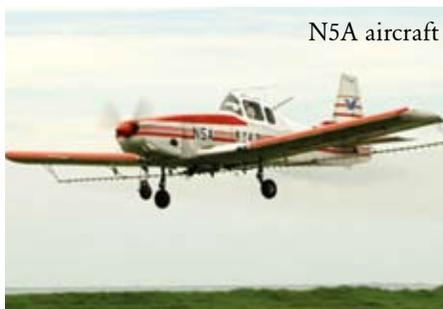
N5A aircraft is designed, developed and produced by Hongdu Group. It is the first multipurpose agricultural and forestry aircraft in China. The aircraft is equipped with an advanced power unit and operation equipment, and can fly in the ultra-low altitude of 3-5 meters high.
