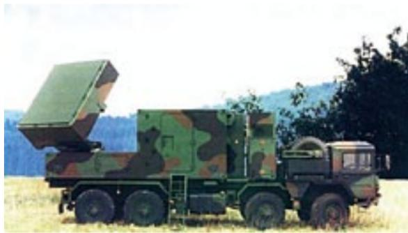
Many of these once state of the art radar systems have also become outdated due to the environment in which they operate in. Increased levels of non static clutter, such as wind farms, increased levels of air traffic densities and new requirements to track smaller cross section targets, like UAV's, all place extra strain on a system that was already operating at the peak of its current abilities.
